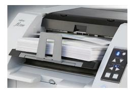
The fi-5950 is equipped with an active stacking tray that automatically maintains a constant height ensuring that scanned documents are always stacked in a neat and orderly fashion..
